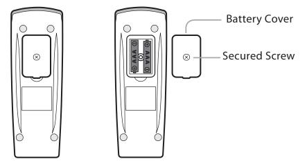
FIGURE 3. Remote Battery Installation
